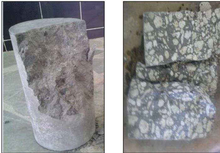
**Figure 4.** Test cylinders of conventional (left) and pumice lightweight concrete (right) after the compressive strength trial.
