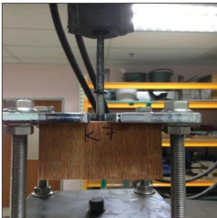
**Figure 13.** The specimen failed in dowel-adhesive
