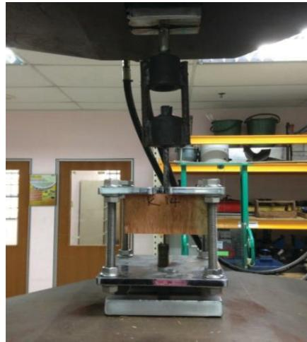
Figure 4. The pull-out test set up
