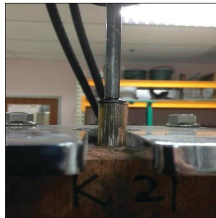
**Figure 14.** The specimen failed in timber-adhesive
