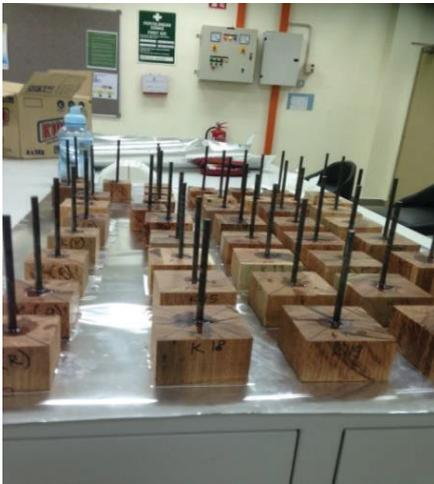
Figure 3. The pull-out test specimens
