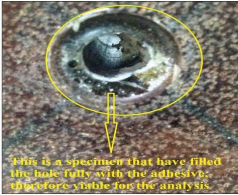
Figure 7. The sample filled with adhesive
