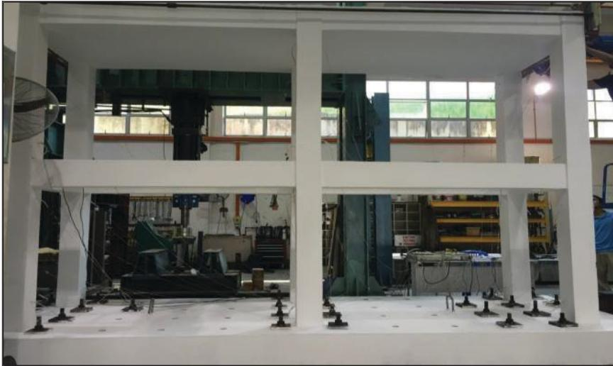
**Figure 2.** The two-bay two-storey moment resisting RC frame
